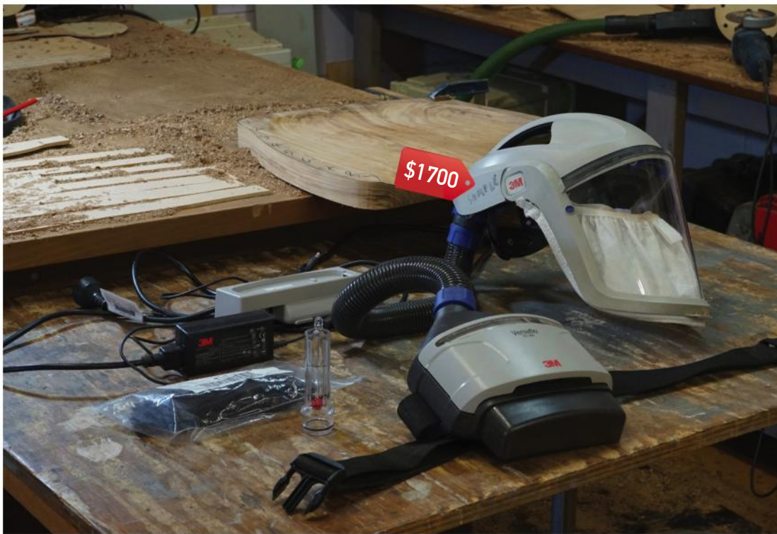
Main: Using the Sundstrom SR580 helmet with SR500 motor. Airflow is 175 and 240 litres/minute.
